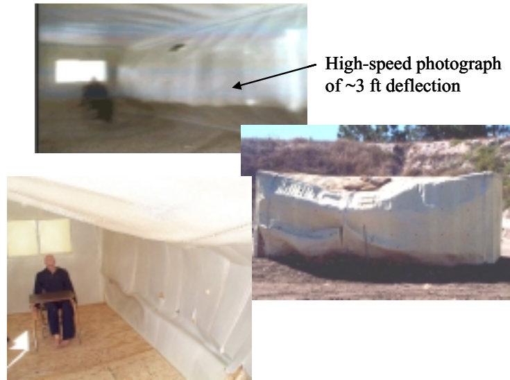
Figure 4. Results of 12 psi Blast Test on Trailer with Polymer Retrofit
